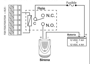
**NOTE:** PGM outputs cannot be completely disabled in installer programming. To completely disable a PGM output, you must remove all wiring from the PGM output.
