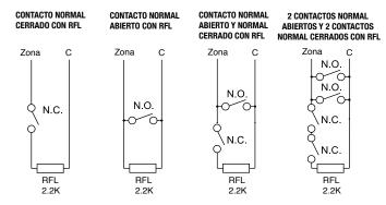
**NOTE:** This is the appropriate connection mode for Normally Open (N.O.) or Normally Closed (N.C.) sensing contacts.
